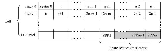
Note: This drive manages alternate spare areas for each cell, which is a set of cylinders. The default value for the number of cylinders is four.
